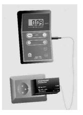
The DGM-1500 has a connector for a mains adapter, allowing it to be used for round-the-clock radiation monitoring. A wall mounting bracket for the meter is available as an optional extra, so the meter can be installed where it is always easily visible. The alarm level is userprogrammable. If the level of the measured radiation exceeds the alarm level a warning tone is emitted (see the section on programming the alarm level).
